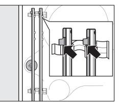
Secure the transit bars to the back of the washing machine. Make sure that the top catch is located above the holder.
